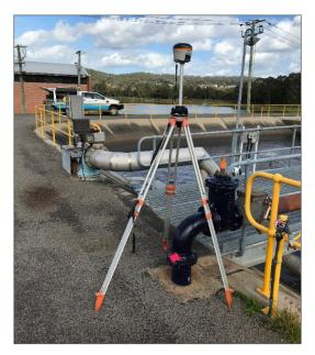
Fig. 2. Hemisphere S321 Smart Antenna.
