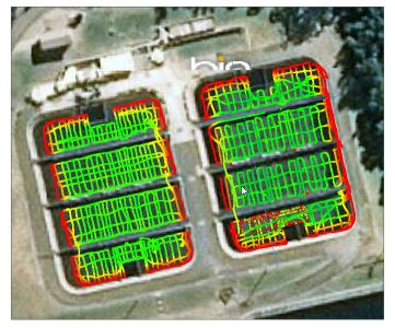
Figure 8: Bathymetric Survey.
